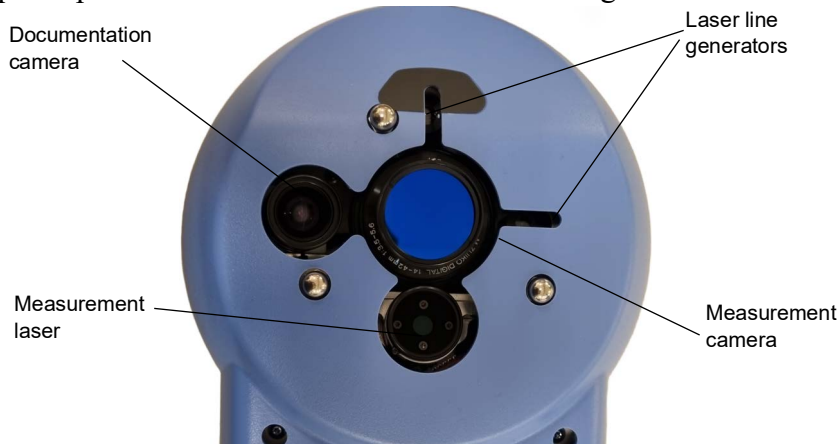
Figure 2-5 Optical parts - view of the PeriCam PSI head from underneath.
