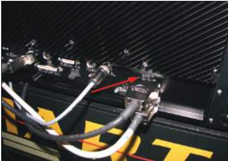
Figure 190: Connection for the image signal cable on the scan head's APD printed circuit board
