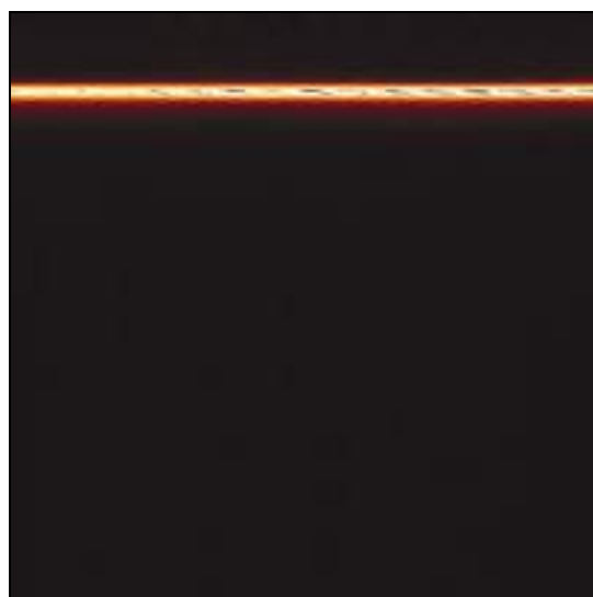
Figure 164: Selection of the FCS measurement position for measurements in solutions: The reflection between the cover slip and the solution must be above the middle of the image.
