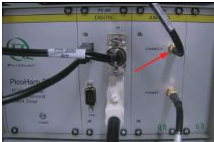
Figure 197: PicoHarp 300 counting unit: At Channel 0, the synchronization cable of the laser used (MP laser or white light laser) is connected
