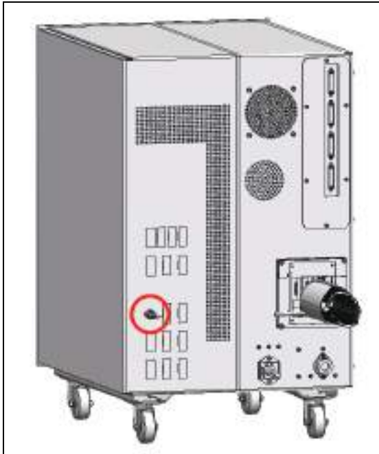
Figure 43: Interlock connector on the compact supply unit
