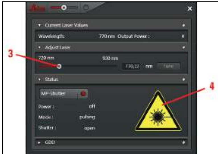
Figure 102: MP Laser Configuration, second shutter open
