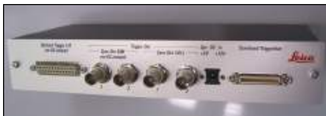
Figure 24: Rear side of the trigger unit
