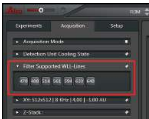
Figure 128: Selection switches to set the laser wavelength and the filter wheel when using the white light laser
