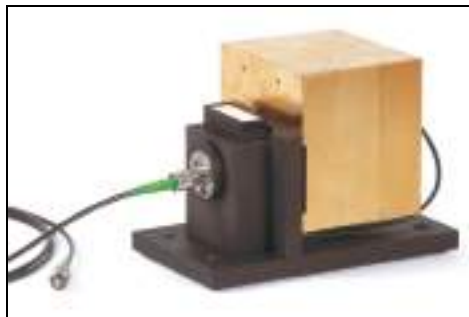
Figure 18: Single-channel PMT detection unit
