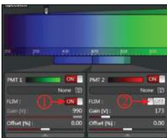
Figure 113: Selecting the operating mode of the internal SP FLIM detectors in Beam Path Settings
