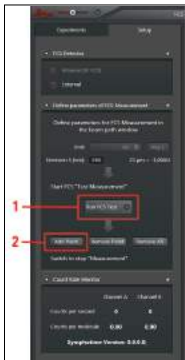
Figure 176: Starting the FCS test and applying the measuring point
