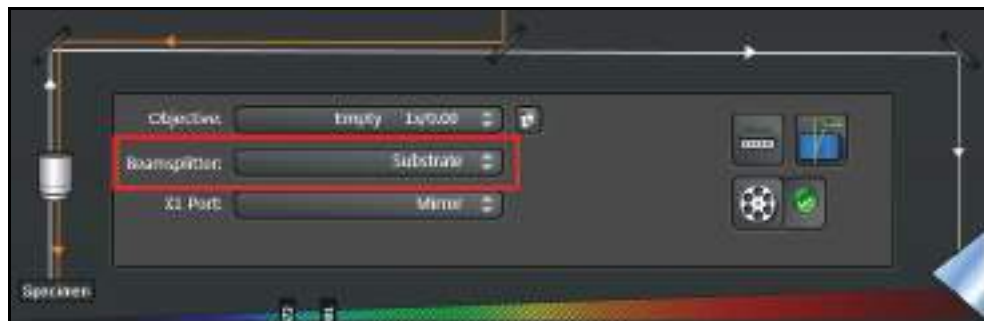
Figure 103: Setting the beam splitter to substrate
