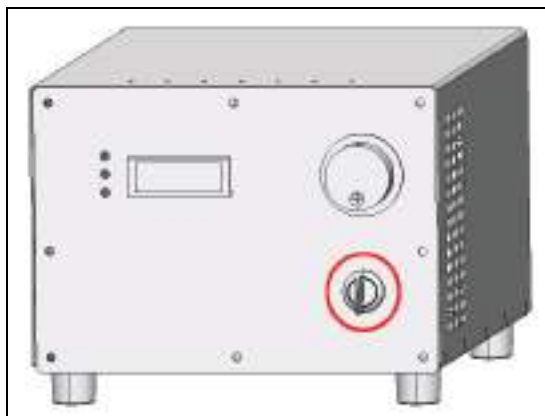
Figure 78: Key switch on the power supply of external UV laser 355
