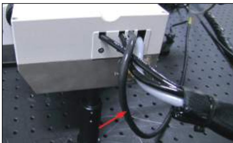
Figure 193: Image signal cable on the HyD RLD, which is attached to the scan head's APD printed circuit board
