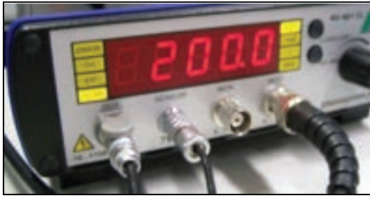
Figure 186: Piezo focus controller
