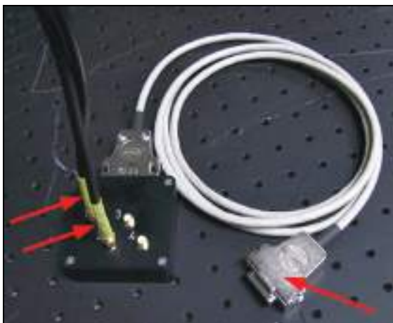
Figure 196: Signal converters to connect the image signal cable of the MPD APDs (SPAD 1 and SPAD 2) to the scan head's APD printed circuit board (see Figure 190)
