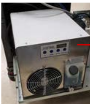
Figure 21.3 Remove the lower rear panel using a hex head wrench to expose the chiller unit
