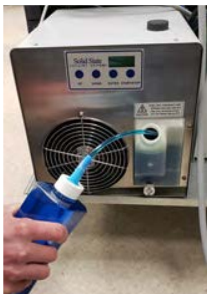
Figure 21.4 Filling the chiller with coolant
