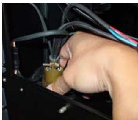
Figure 22.6 Disconnecting the electrical connector and inserting the unlocking key into the key receptacle
