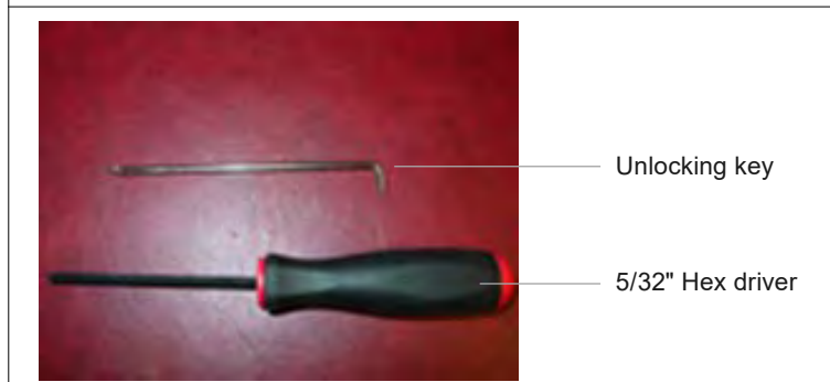
Figure 22.4 Tools required for deactivating the solenoid lock
