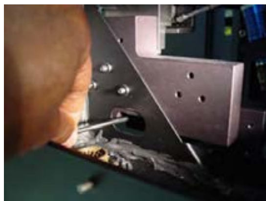
Figure 22.6 Disconnecting the electrical connector and inserting the unlocking key into the key receptacle
