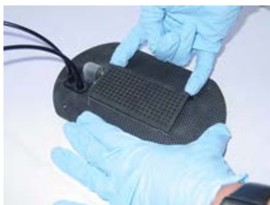
Figure 7.8 Removing the Bed from the Single Mouse Manifold/ Stage
