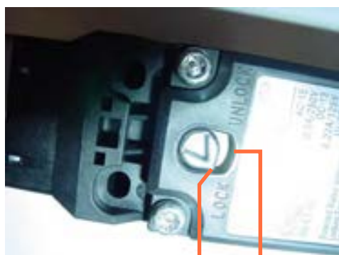
Figure 22.7 Key receptacle and solenoid unlocking key
