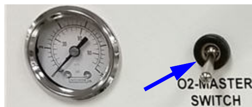
Figure 28. O2 Master Switch
