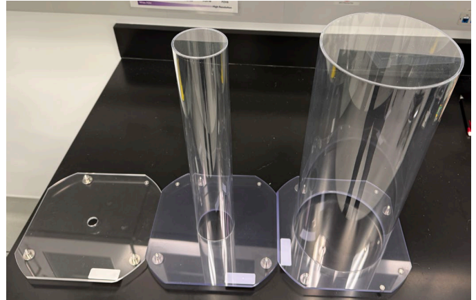
Figure 4.5: Bore covers from right to left. 86mm FOV bore cover, 18 mm FOV bore cover, 8mm FOV bore cover
